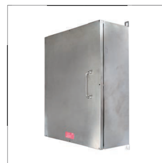
Stainless Steel Terminal Box Series: EX-PD62 Voltage: Max AC1100V Current: 24A/32A/41A 57A/76A/11 5A/126A/ 184A/218A/265A/350A Degree of Protection: IP66 Zone 1,2, Zone 21,22
