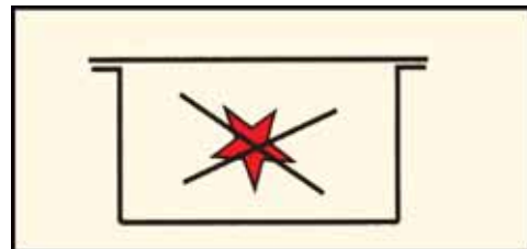
Principle of the type of protection "increased safety"
