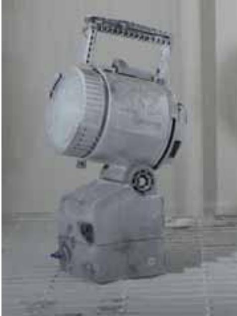
Explosion protected searchlight inside the dust test chamber
