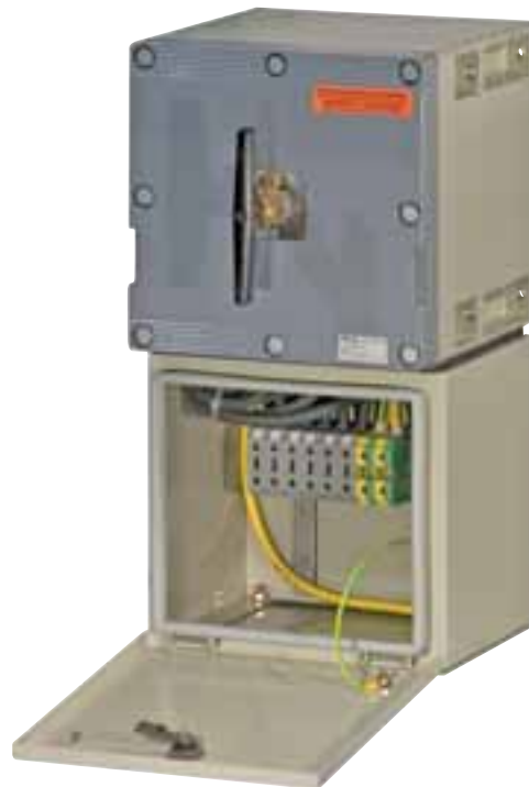
Rotary switch in flameproof enclosure of the series GHG 64 with flat joint and flanged-on Ex-e connection box for indirect connection
