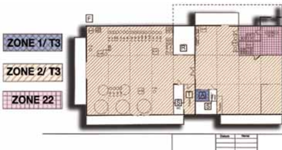
Zone classification example: Explosion-protection zone plan for explosive gas and dust atmospheres
